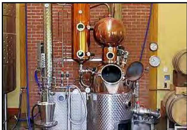
Hand-crafted copper Mueller still at Merridale
